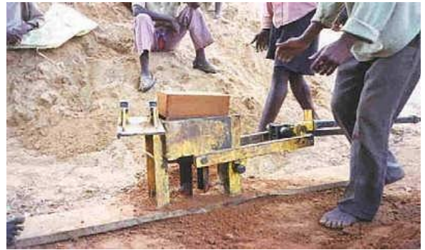
Above: A Cinva-Ram hand press for making compressed earth block.
